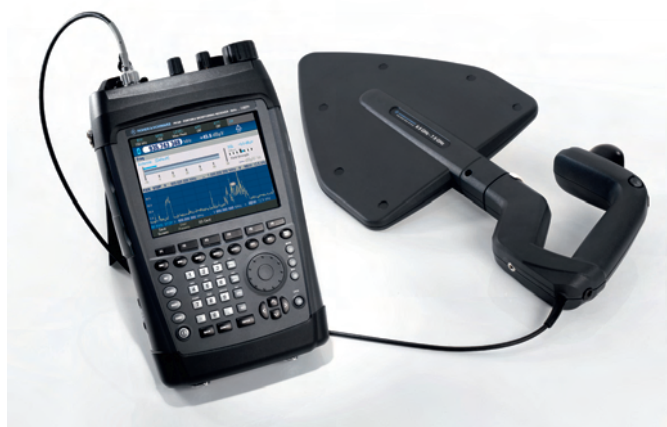
R&S®PR100 with R&S®HE300 active directional antenna: The antenna comes with three modules that cover the frequency range from 20 MHz to 7.5 GHz (can be expanded to 9 kHz with optional HF module). The preamplifier is accommodated in the grip piece.
