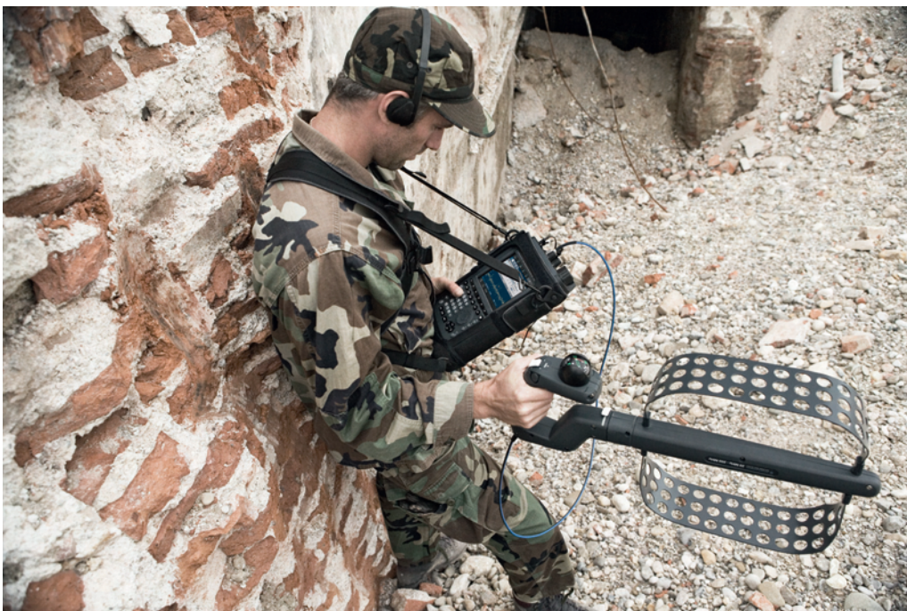
Tracking telltale signals by means of the R&S®PR100 and the R&S®HE300 active directional antenna
